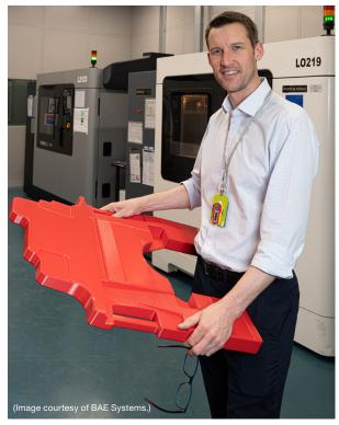
Greg Flanagan, pictured with a 3D printed Typhoon cockpit floor cover, says that Stratasys FDM additive manufacturing helps BAE Systems meet its overall company objectives to reduce costs and time-to-market.
