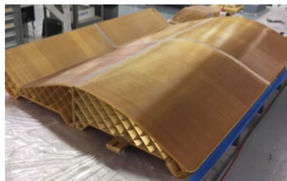
Figure 15. Assembled 4-piece FDM cabinet headliner lay-up mold.
