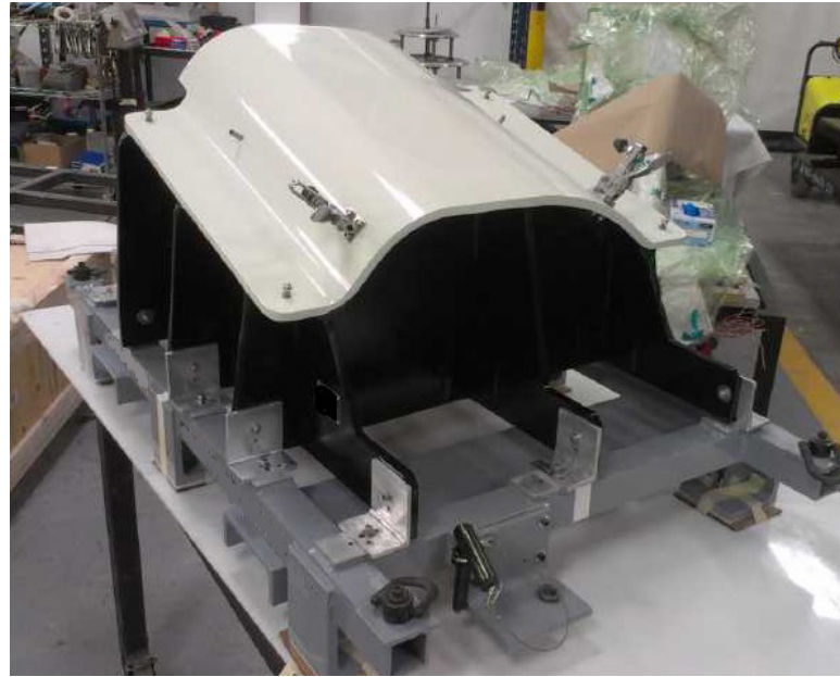
Figure 11. FRP machining fixture for the speaker box panel.
